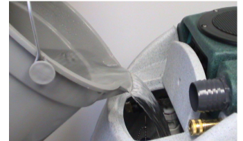
Pour 2 or 3 gallons of clean water into Solution Tank
